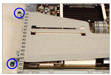
Figure 22: Removing the riser card holder
